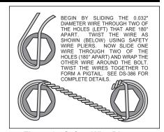
Figure 3. Safety Wire Diagram
