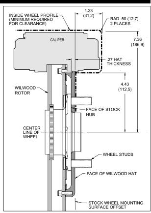
Figure 2. Wheel Clearance Diagram
