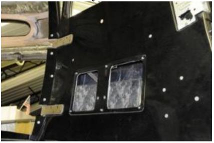
34. Installation of the bottom part of the doors was done using horizontal pieces of HushMat.
