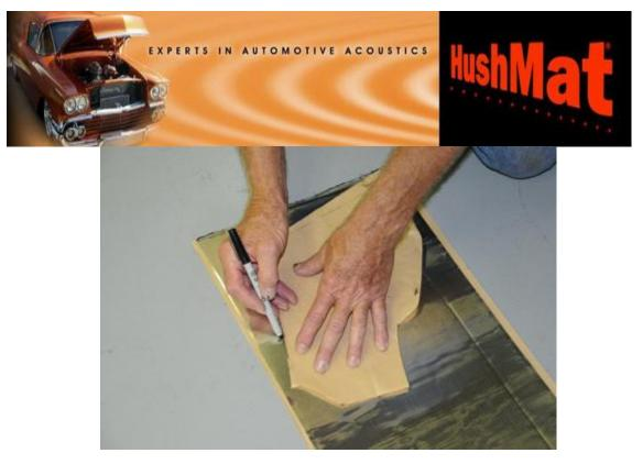
18. After cutting out the drawing made on the backing paper, the pattern is placed on another sheet of HushMat Ultra and traced with a felt tip pen.
