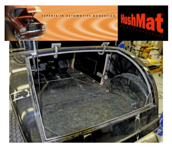
3. The trunk area was open as well so installation was easier. There is no special preparation of the surface needed before installing HushMat. No acetone or other solvent cleaning of the surface was required with HushMat. I vacuumed the complete inside of the body to remove any dirt that was loose on the floor.
