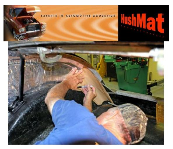
17. The sides of the body were the next area's to cover. The open flat sections were covered first and then patterns were made again using the waxed backing paper peeled off of prior sheets. Draw out the area by pressing the paper into the section to be covered and trace it out with a felt tip pen.
