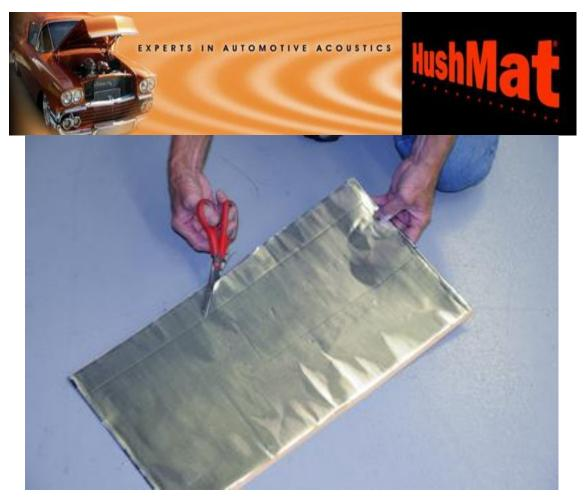
13. Now simply cut out the traced line on the HushMat Ultra sheet using the scissors.
