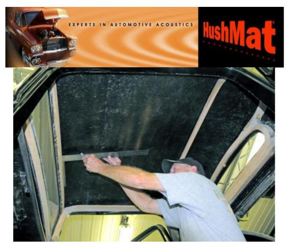
6. After locating the center of the roof area, a straight edge and felt tip pen were used to draw a line on the roof. I found this to be a good way to decide how I was going to install the HushMat Ultra sheets and get the most material use without waste. The HushMat Ultra sheets are 12X23 inches.
