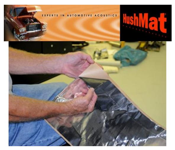
8. You simply peel the wax backing paper off of the HushMat Ultra sheets as shown here. The sheets adhere very nicely to the surface. A good idea is to think ahead of the process and trial fit the pieces before peeling the backing paper off and pressing into place.
