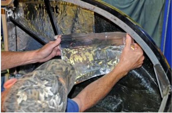
19. This piece is now easily installed in the area it was made to fit into. The HushMat is so very easy to install and really sticks to the surface well. On compound curves like this area, it forms easily and lays down very nice.
