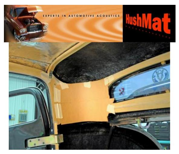
10. The wood frame areas on both sides of the rear window were going to be a problem, so I used a scrap piece of soft cardboard that conformed to the opening. I then used masking tape to hold it in place over the opening.
