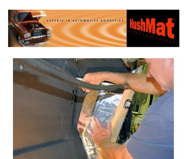
23. The front kick panel area on the passenger side is installed after making a pattern as described earlier.
