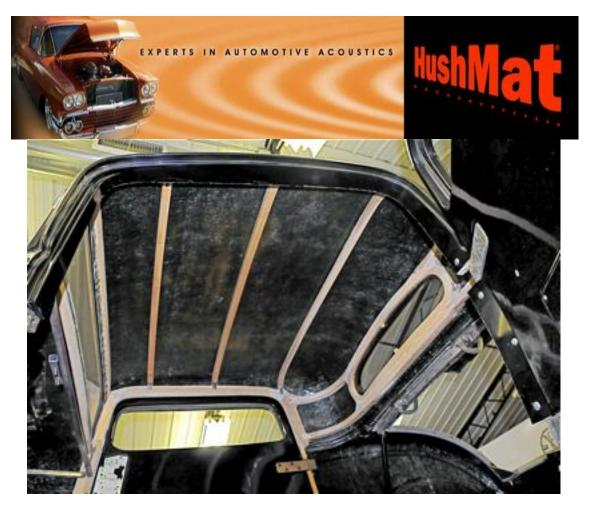
4. The roof in the coupe has wooden bows for attaching a headliner. I unscrewed them from the wood frames around the doors, and removed them for ease of installing the HushMat sheets.
