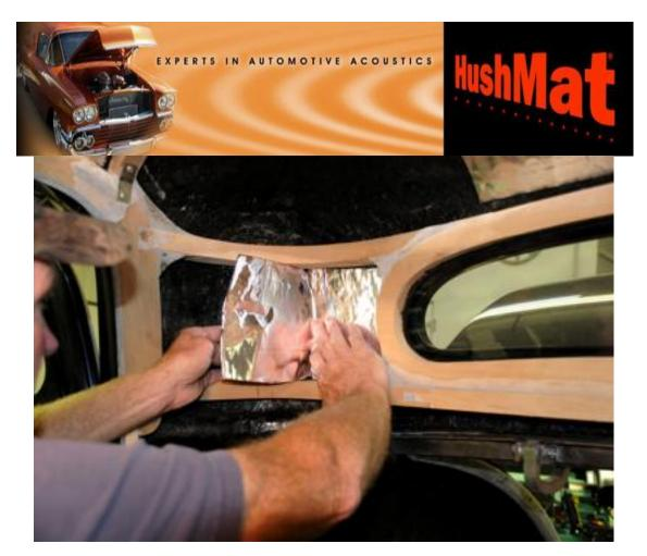
13.The piece of HushMat just cut out can now be easily placed into the tight area next to the rear window as shown.
