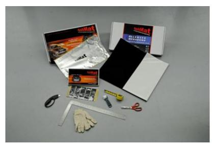
1. These are the HushMat products and suggested tools needed to install Hushmat in any type vehicle. A tape measure, scissors, utility knife, straight edge, and small hard roller are essential, but the gloves are optional. The edges of the foil can cut your hands so the gloves may be helpful. I personally didn't need them and had no problems.
