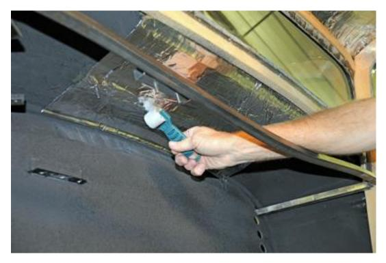
22. Here the sheet is rolled down using the small roller
