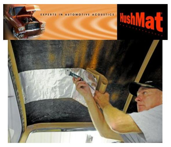
9. The decision was made to run the sheets longitudinal with the marked centerline. Here the small hard roller is being used to roll the sheet down as the backing paper is removed.
