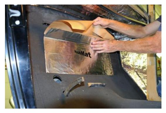
25. The next area to cover is the firewall. Again I started in the center of the firewall and filled in the sides as needed. Simply mark, press, and peel, it's that easy!
