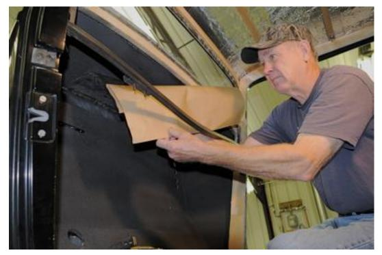
21. The next area to be covered is under the dash/cowl on a '32 Ford. The underside of the cowl is exposed to the outside, so heat and sound deadening is important. This first sheet was placed in the very center under the cowl.
