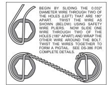
Figure 4. Safety Wire Diagram
