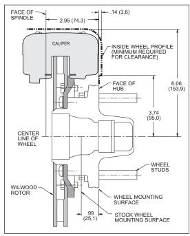
Figure 1. Wheel Clearance Diagram
