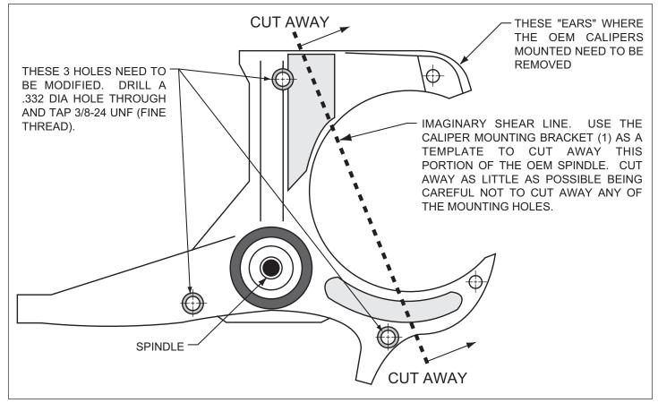
Figure 2. Typical Steering Arm / Spindle Modifications
