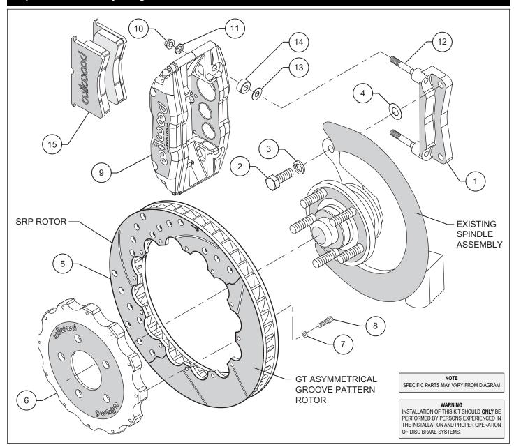
Figure 1. Typical Installation Configuration
