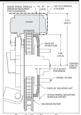
Figure 2. Wheel Clearance Diagram
